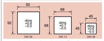
DIN 48 can be slot mounted using the standard fixing clip.
