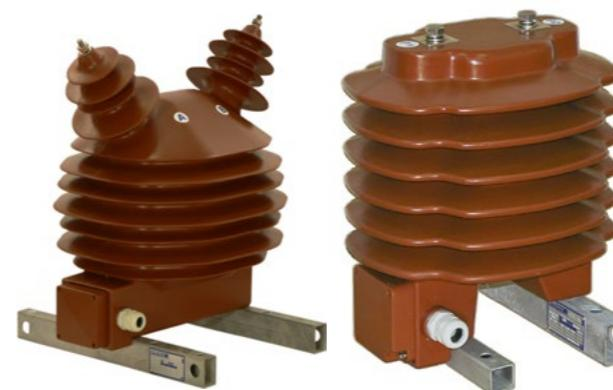
These instruments current and voltage transformers are intended for measuring and protection of high voltage distribution systems of the indoor as well as outdoor type. These instruments transformers are intended for the voltage system from 3,6 kV up to 40,5 kV. The transformers comply with requirements of IEC 60044-1, IEC 60044-2, GOST 1983-89 and DIN 42600/1983.
