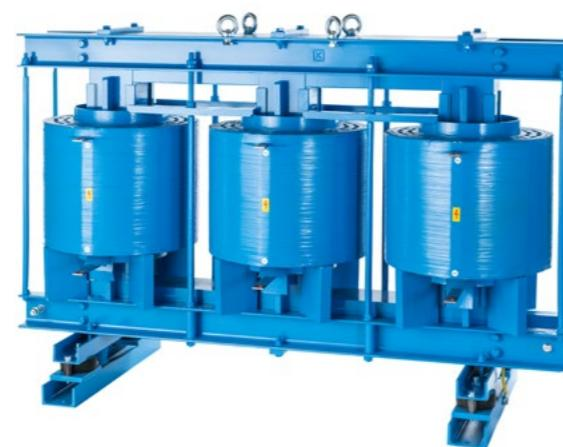
Standard design is intended for detuned capacitor banks. Reactors have high linearity, low losses and minimal noise. Inductance is fixed to the exact value with tolerance of  $-1/+3\%$ . Reactors are designed for capacitors at 7200 V (grid 6000 V) and 12000 V (grid 10000 V), 50 Hz and tuned to resonance frequency of 189 Hz. Reactors are wound on Fe core with insulation class „B”.
