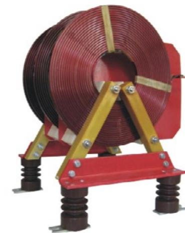
Standard design is intended for high voltage capacitor banks as protection against very high peak currents during switching (inrush current). Max rated voltage 40 kV, max rated current 250 A. Standard rated voltage 7,2 and 12 kV. Insulation class is „F”.
