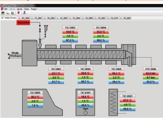
Extruder Control System - view of a single control zone.
